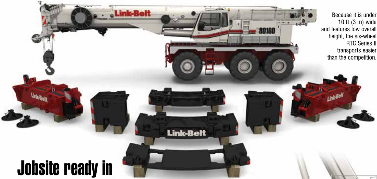
Because it is under 10 ft (3 m) wide and features low overall height, the six-wheel RTC Series II transports easier than the competition.
