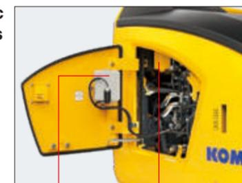
Washer tank Auxiliary hydraulic circuit return filter
